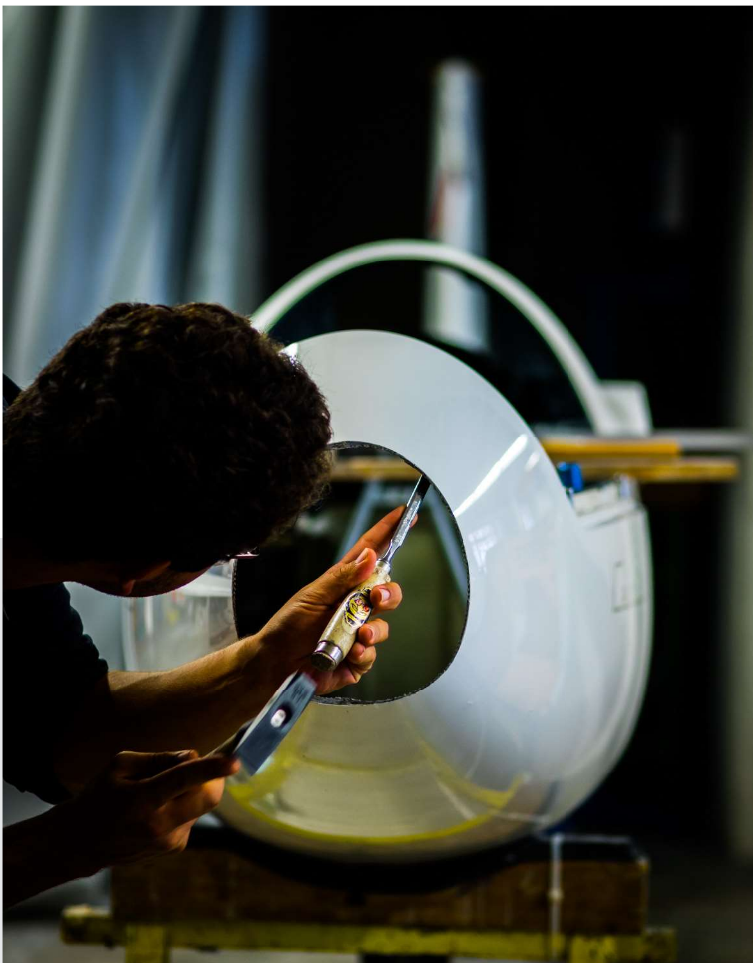
Installation of the FES system in the fuselage frame needs extra care and precision. Schempp-Hirth Kirchheim.
